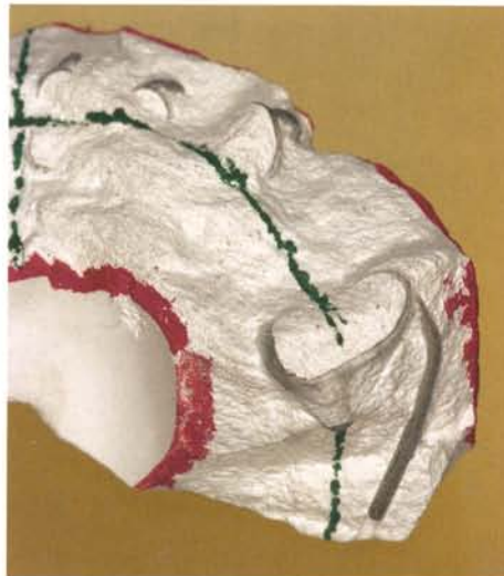
Fig. 41. The precise centering of the metal and the heat vent becomes visible during devestment. If you note these details and also leave the cast to cool slowly, you can be sure of a satisfactory result.
