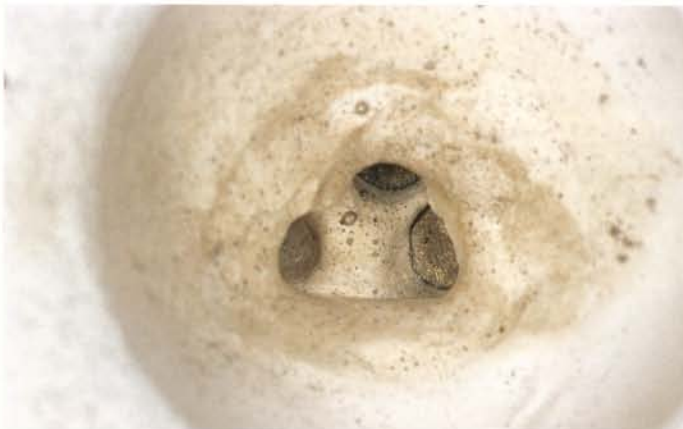
Fig. 40. Detail of the casting flask after pouring. Sprue staining is uniform and there is no metal cone, indicating that the quantity and quality of precious metal were properly measured.
